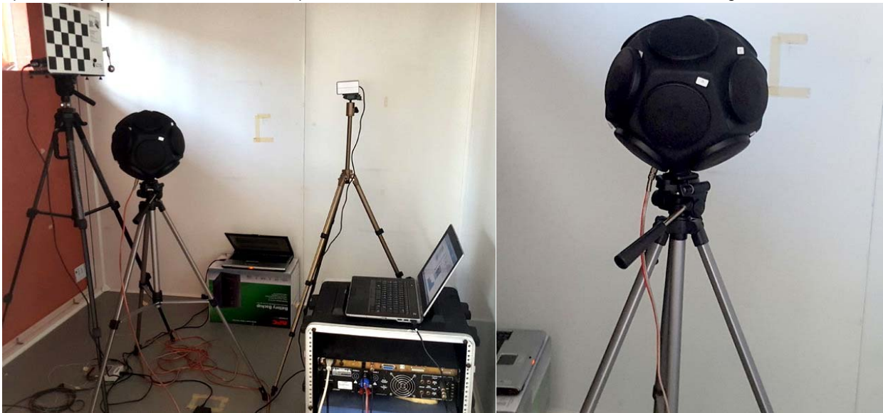
Figure 9: Experimental setup for sound intensity measurement at the inner side of the mock-up panel. From left to right: SoundBrush probe and calibration board, 12-speaker spherical source, tracking camera, control laptop running Siemens SoundBrush software with amplifier
