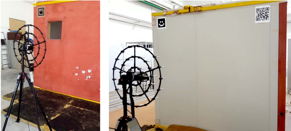
Figure 13: Microphone array measuring the sound pressure from the different panels of the Dragados-UNIVPM mock-up. Mineral wool panels were placed on the floor in order to suppress parasite reflections
