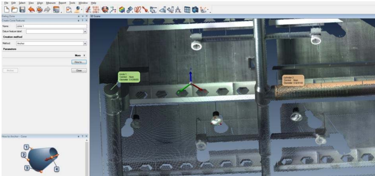
Figure 31: Cone adjusting for lamp 3D modelling.
