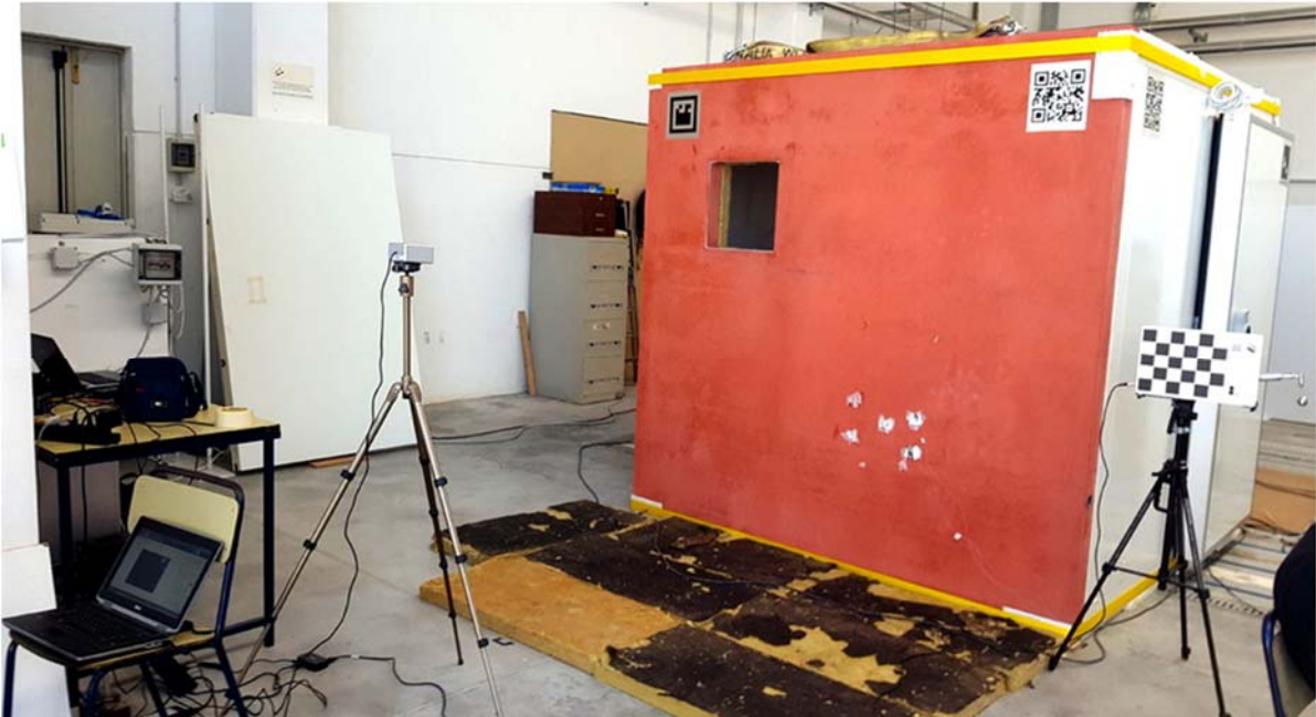
Figure 10: Experimental setup for sound intensity measurement at the outer side of the mock-up panel
