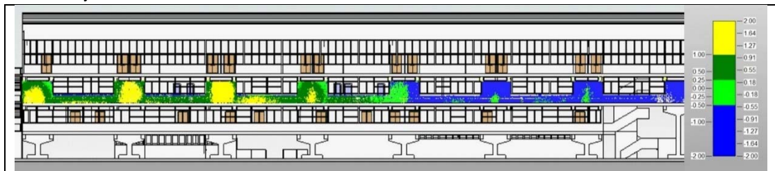
Figure 53: Result of deviation analysis by "pick face" method
