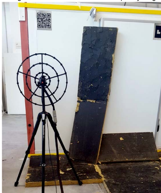
Figure 14: Microphone array at the side of the Dragados panel for acoustic leakage identification. Mineral wool panels were placed on the door and floor sealings in order to suppress the sources of noise originating thereupon, so as to correctly identify the noise source due to the imperfect sealing of the Dragados panel, introduced intentionally for this test. Note: the array position in the photograph does not correspond to the final configuration
