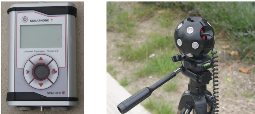
Figure 4 Ultrasound generator and sound source. [Source: Insiter]
