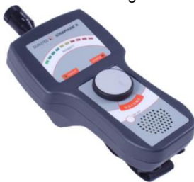
Figure 5 Sonotek ultrasound receiver. [Source: Sonotek]
