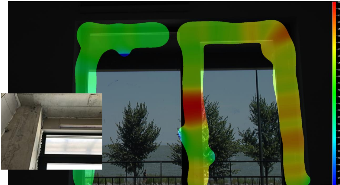
Figure 25 Ultrasonic recording [Source: Gevelscan Ultragraphy ( www.ultragraphy.com )]
