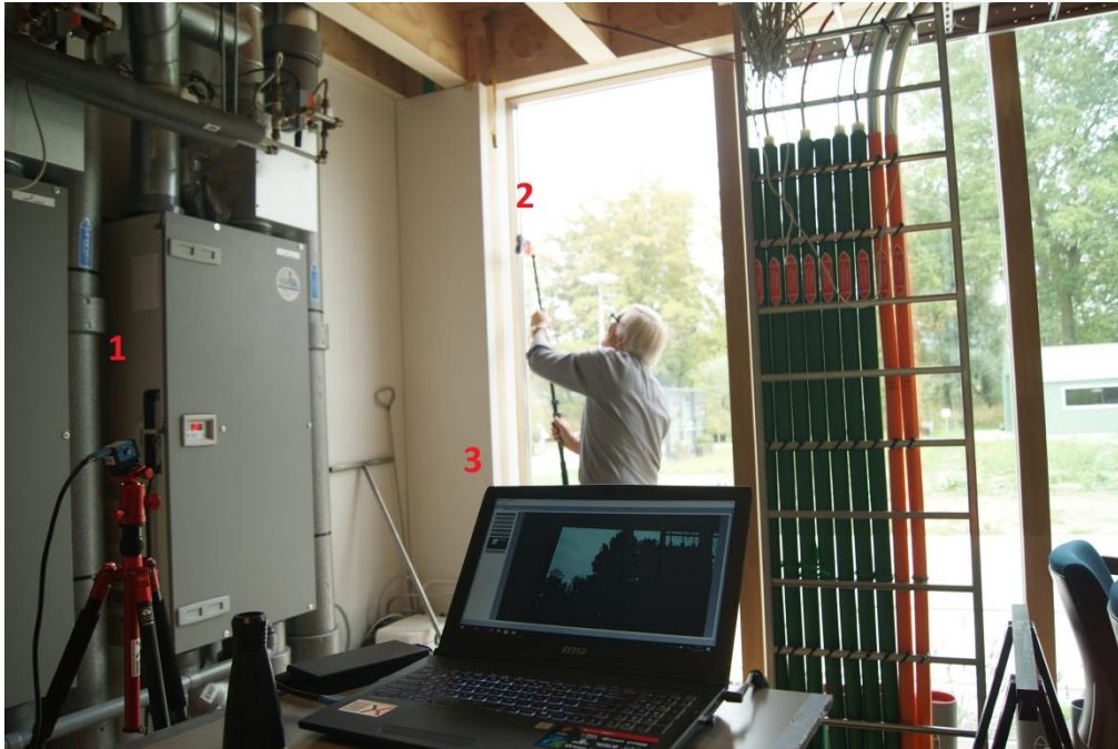
Figure 10 Setup Ultra Photography measurement: 1. Camera 2. Receiver 3. Laptop with software. The Ultrasound sound source is outside and is not visible in this photograph. [Source: Insiter]
