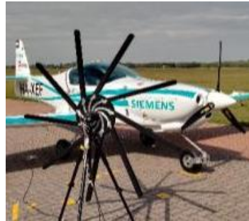
Sound source localisation on the engine of an aerobatic electric plane. (Ground setup using Sound Camera)
