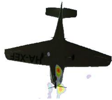
Sound source localisation on an aerobatic electric plane. (Fly-over setup using a purposely-built 100-microphone ground array)
