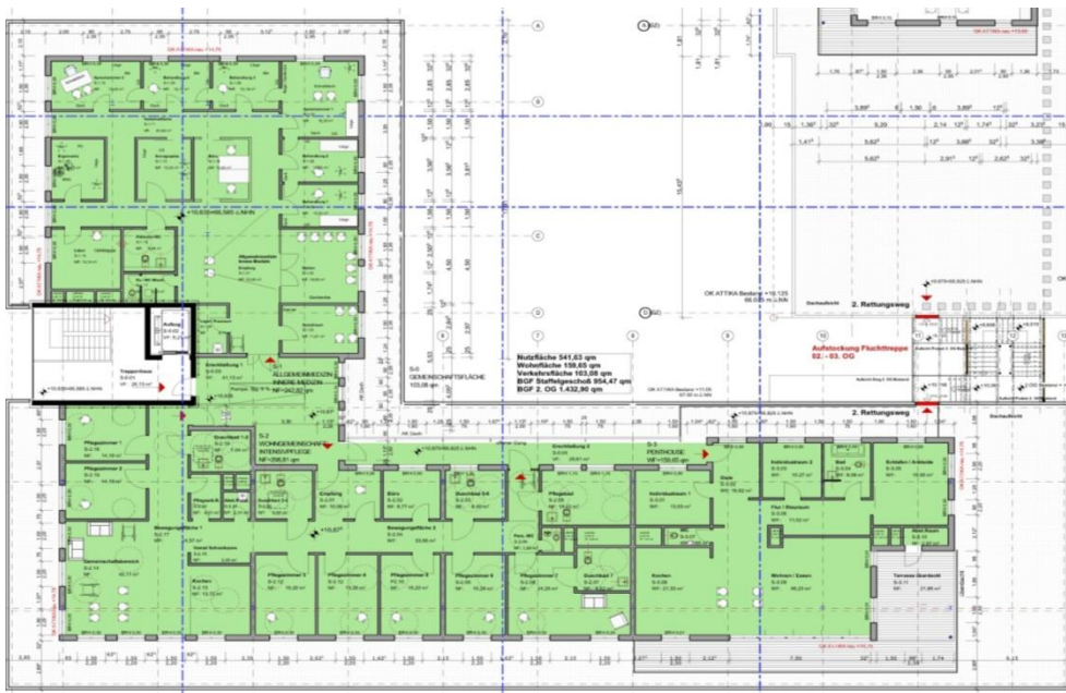
Figure 3: floorplan planned rooftop extension (green)
