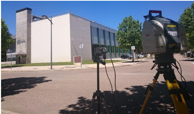
Figure 18: 3D laser scanning of CARTIF-3 as example of energy efficient building made of pre-fab components
