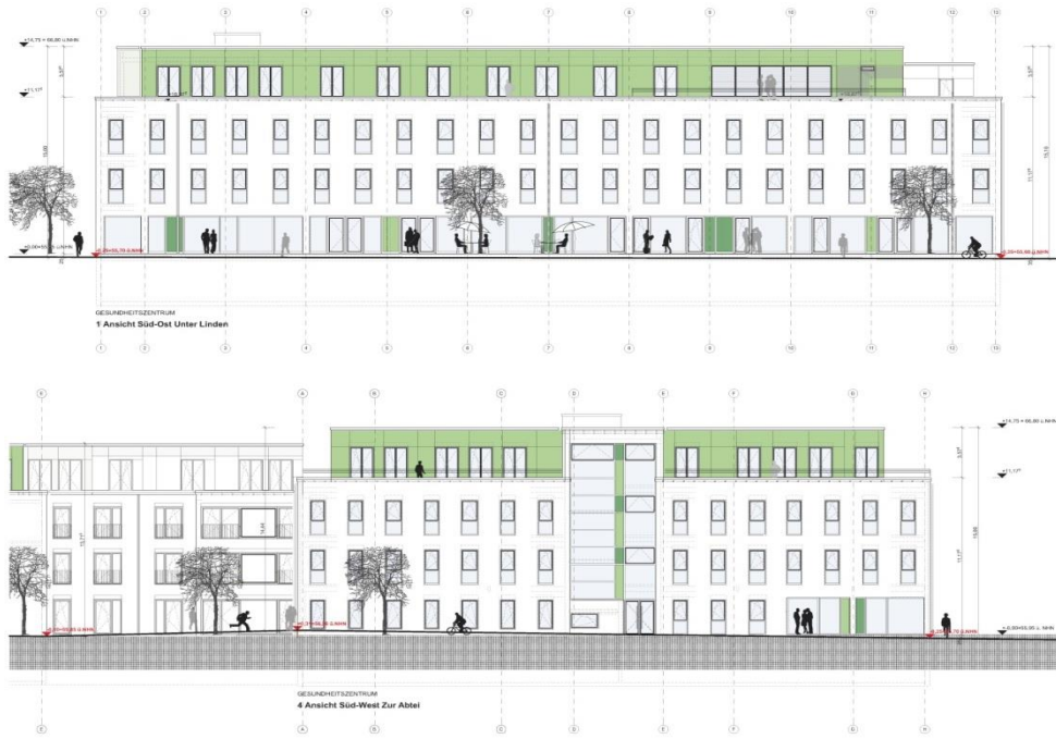
Figure 2: elevations planned rooftop extension (green)
