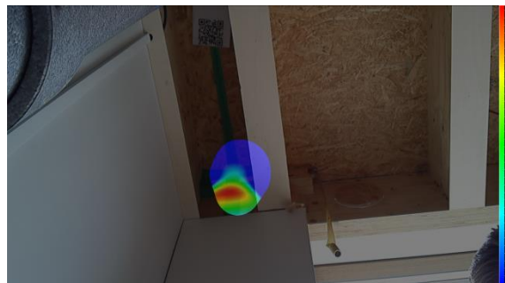
Figure 54: Misinformation of air leak caused by sensitivity of the receiver for knocking against hard surfaces
