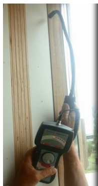
Figure 48: Test setup with receiver which makes the ultrasound audible (ultrasonic)
