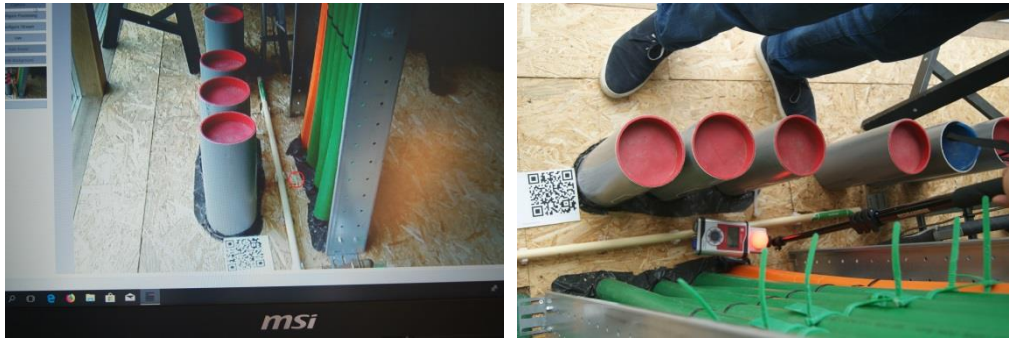
Figure 51: During measurement the receiver is seen by the camera and plotted on the photo with a red circle
