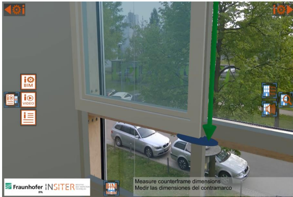
Figure 117: INSITER BIM-based Self-Instruction AR app visualizing self-instruction information for different BIM objects
