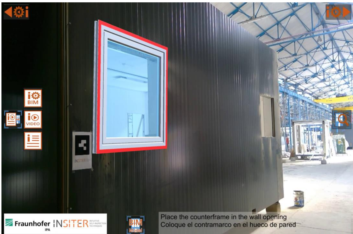
Figure 194: INSITER BIM-based Self-Instruction AR App screenshot - Visualizing self-instruction information for BIM elements and to be installed window components for the DRAGADOS Use Case Demo in Seville on tablet computers
