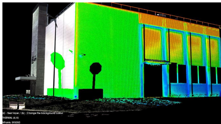
Figure 146: Point cloud with thermographic overlay usable into REVIT
