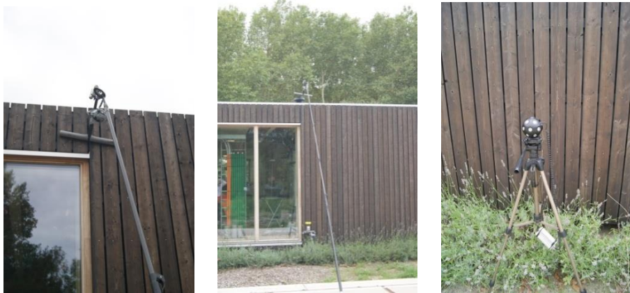
Figure 47: The transmitter and generator were placed near the places to be investigated for airtightness. For the cable entry through the floor the transmitter and generator were placed under the module.
