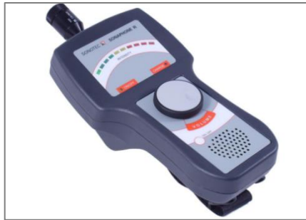
Figure 45: Ultrasonic receiver used for first quick inspection
