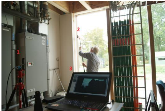
Figure 49: Test setup with ultrasonic receiver (2), camera (1) and laptop (3) (ultragraphic) which makes the ultrasound visible (ultragraphic)
