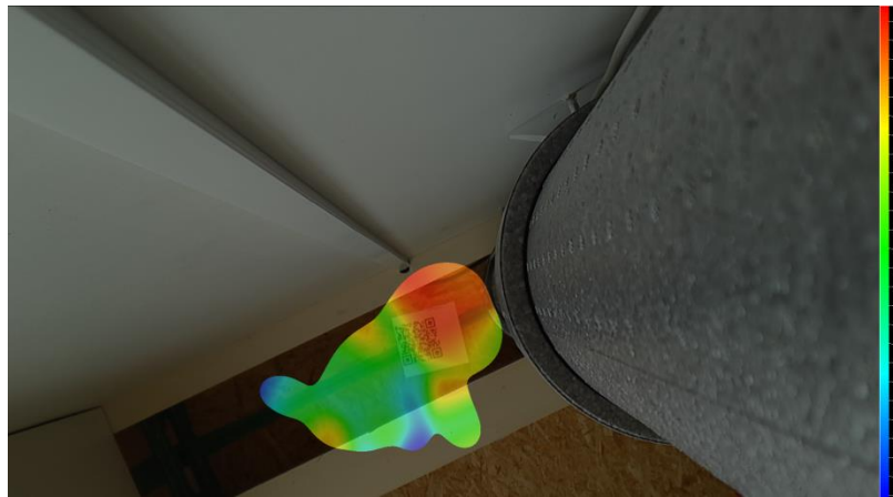
Figure 62: Ultragraphic of the duct entry
