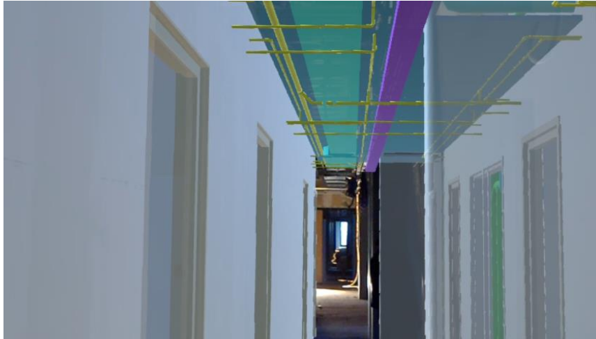
Figure 102: INSITER HoloLens BIM-based Mixed Reality App – On-Site Demonstration with complete BIM model (without ceiling, MEP/HVAC party hidden by digital wall elements)
