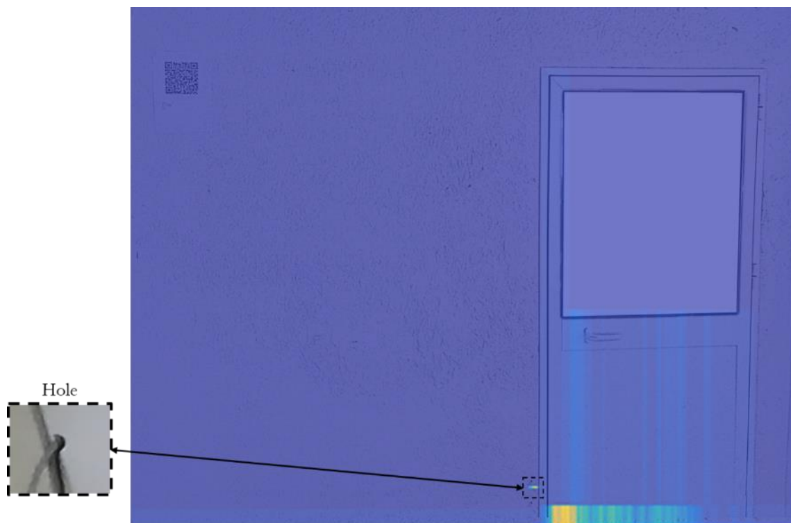
Figure 185: Ultrasonic signal superimposed to Wall 2 picture
